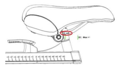
3. Make sure that the comfort sport saddle is fixed in a level horizontal and vertical position. Use the ratchet to tighten the nuts with at least 25Nm of torque on both sides to make sure the saddle is secure.
