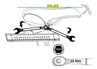
4. Briefly ride the cycle to make sure that the seat is securely in place. If the seat moves at all, tighten the nuts further.
